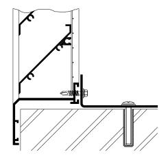
Fixing style for small to medium sized louvre panels. Brackets are of 1.6mm galvanised sheet steel folded but undrilled. Screws and bolts supplied by others. Brackets should be affixed direct to rear of louvre frame by self-tapping screws. The quantity of brackets is at the factory's discretion (minimum 4 No.).
