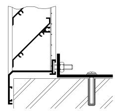
Fixing style for the larger sized louvre panel with either flanged framing or recess style frame. Specially formed 'Tee Bolts' traverse within the track at the rear of frame. Bolts and brackets supplied but quantity at the factory's discretion.
