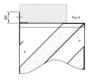
The loose flange option can be used as a fixing method as shown in figures A and B, cosmetically to mask irregularities in the builders work opening, or to perform both functions as depicted in Fig.C. In any event the flange component is finished to match the unit and is furnished undrilled unless otherwise requested. For large sized units the flange is supplied in sections.
