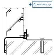
Fixing style '+4' is ideal for small to medium sized louvre panels. Brackets are of 1.6mm galvanised sheet steel folded but undrilled. Screws and bolts supplied by others. Brackets should be affixed direct to rear of louvre frame by self-tapping screws. The quantity of brackets is at the factory's discretion (minimum 4 No.)
