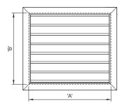
Size is expressed as 'A' x 'B' and relates to the nominal opening size into which the louvre is to be offered. A manufacturing size reduction tolerance is provided. Dimension 'A' (Width) should be stated first followed by dimension 'B' (Height).
