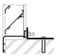
Fixing style '+2' is intended for the larger sized louvre panel with either flanged framing or recess style frame. Specially formed 'Tee bolts' traverse within the track at the rear of frame. Bolts and brackets supplied but quantity at the factory's discretion.
